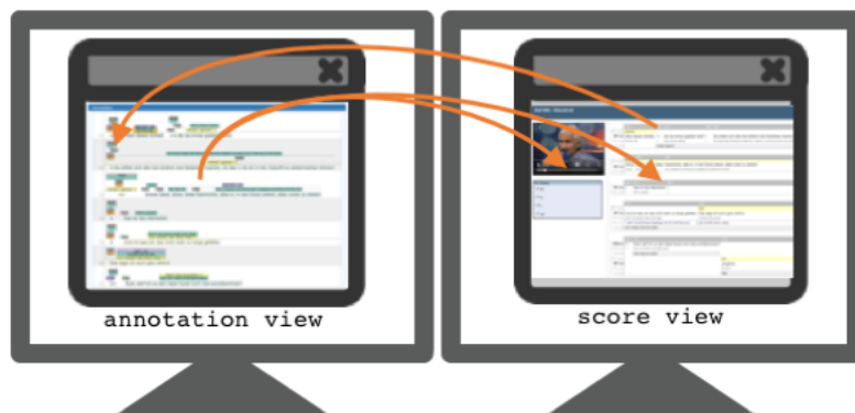
Figure 6: Schematic overview of the synchronization feature and the intended application operation mode: Two monitors, where one holds the browser window of the annotation view and the other holds the browser window of the score view, synchronized by clicking on the respective time markers.
